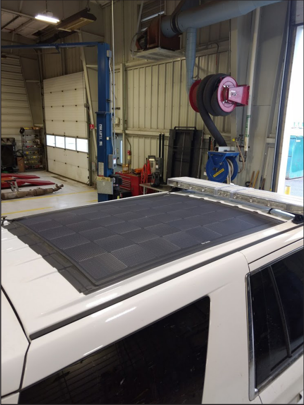
Solar panels placed on the roof of a Chevrolet Tahoe are part of the no-idle HVAC system being tested by INL Transportation Services and the Sustainable INL program.
